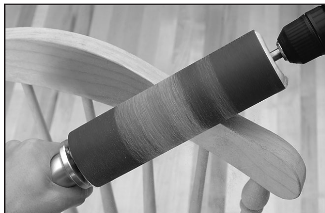
Figure 2. Pneumatic drum sander in action.
