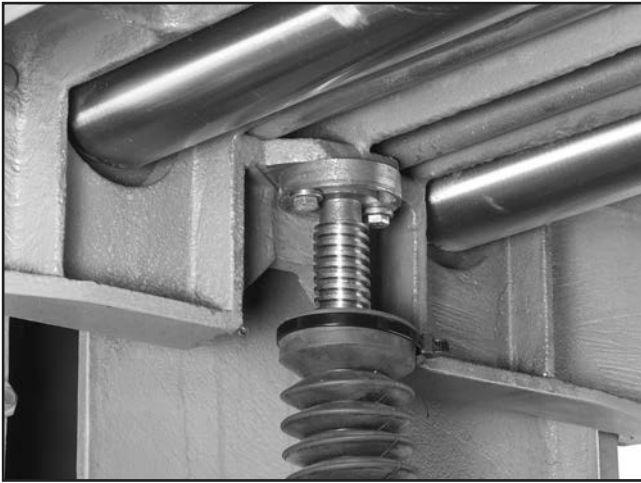
Figure 14. Column adjustment flange underneath table.
