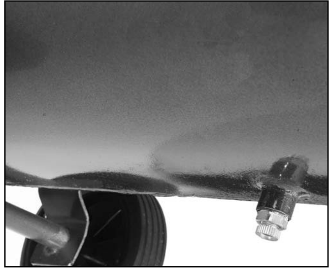
Fig 6. Typical location of drain cocks.
