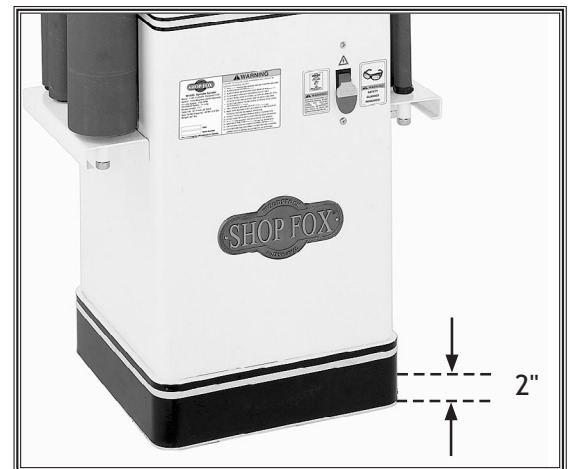
Figure 4. Example of 2" high band on machine base.
