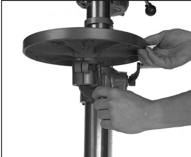
Figure 6. Installing the table.
