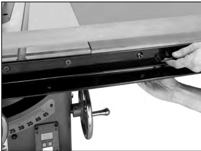
Figure 18. Aligning main extension table.
