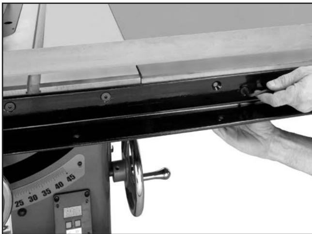
Figure 7. Aligning main extension table.
