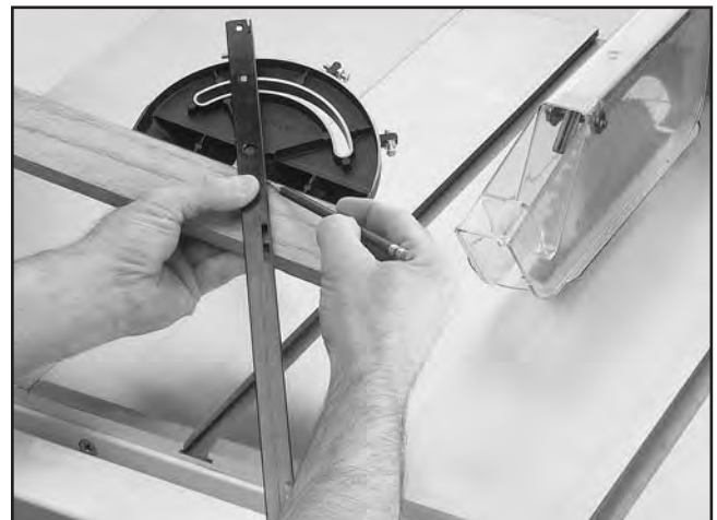
Figure 61. Example of marking miter line.
