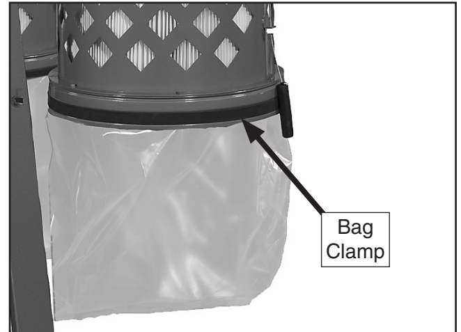
Figure 29. Canister filter collection bag installed.
