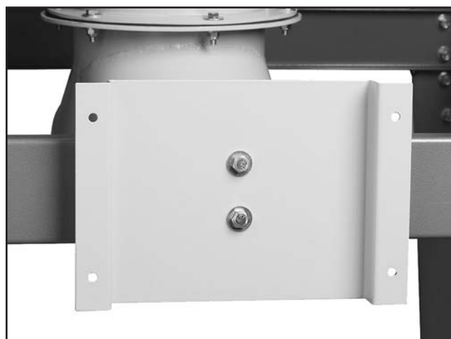
Figure 49. Model G0638 control box bracket mounted.
