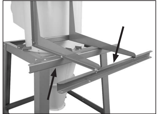
Figure 33. Long brace supports attached.
