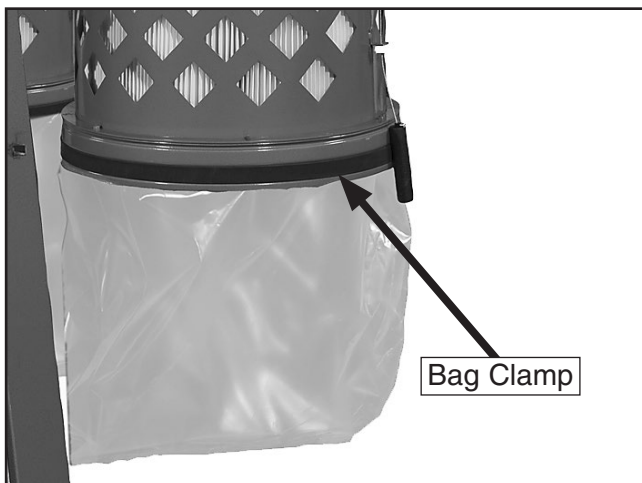
Figure 36. Canister filter collection bag installed.
