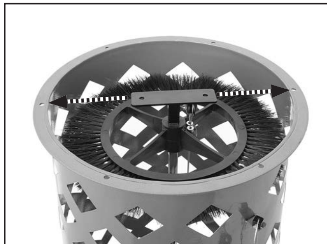
Figure 93. Filter brush base aligned with assembly fastener holes.
