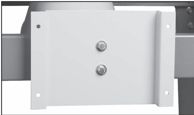
Figure 44. Model G0638 control box bracket mounted.
