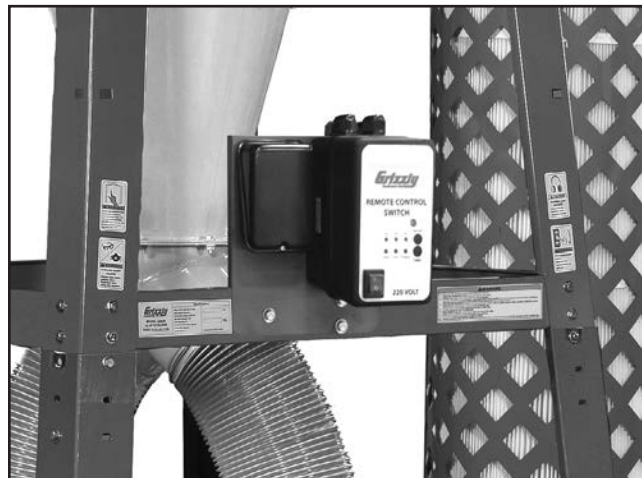
Figure 48. Model G0637 control box mounted.
