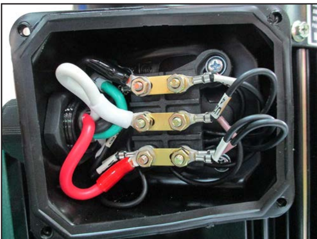
Figure 95. Model G0637 motor wiring (220V).
