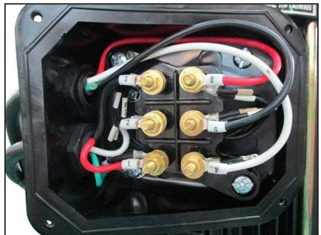
Figure 100. Model G0638 motor wiring (220V).
