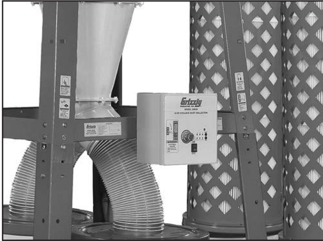
Figure 50. Model G0638 control box mounted.
