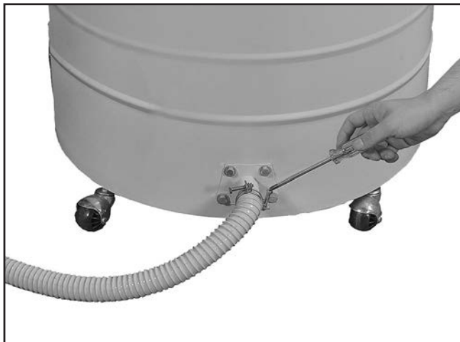
Figure 46. Connecting the vacuum hose.
