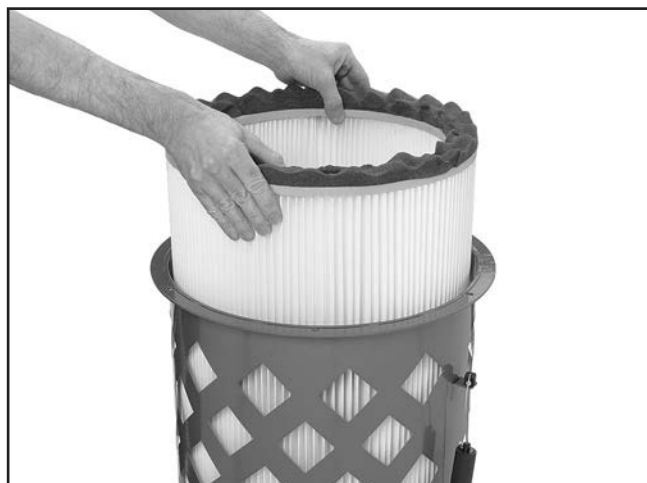
Figure 92. Removing the filter from the canister assembly.
