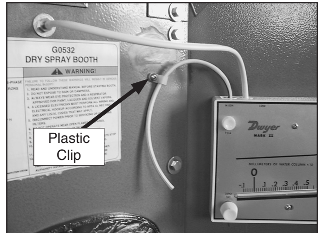
Figure 26. Tubing secured with clip.
