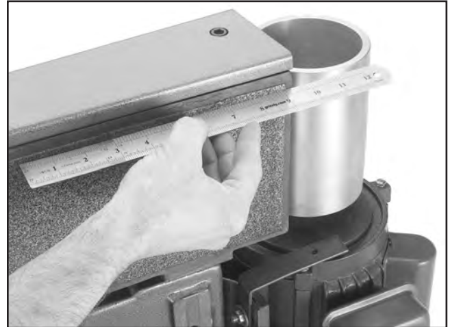
Figure 68. Checking gap between top of platen graphite and drive roller.
