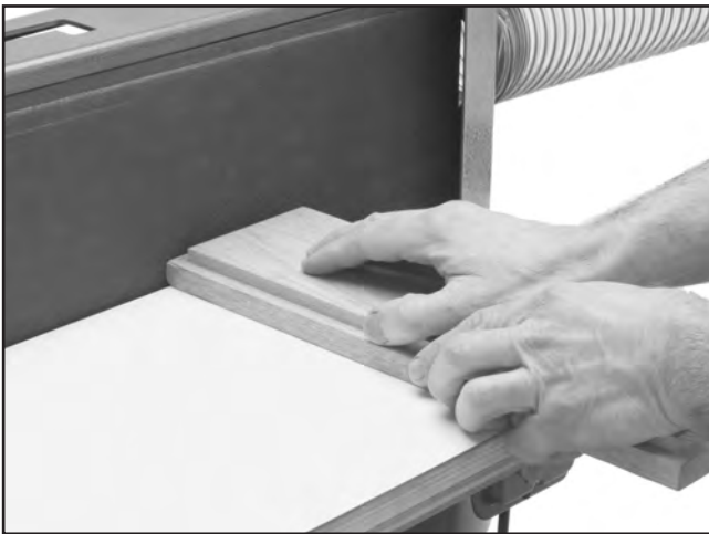
Figure 43. Typical end sanding operation.
