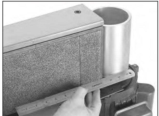
Figure 69. Checking gap between bottom of platen graphite and drive roller.
