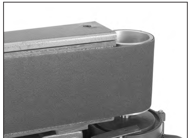
Figure 38. Sanding belt even with top of drive roller (dust port removed for clarity).
