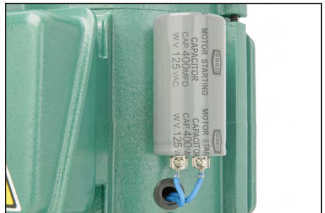
Figure 74. Start capacitor wiring.
