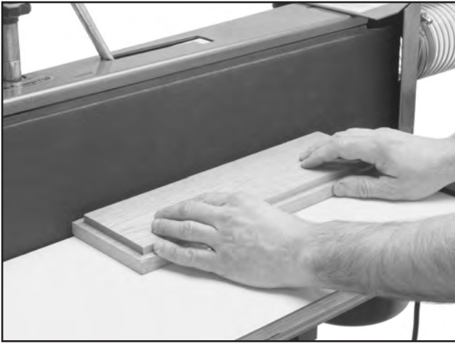
Figure 42. Typical edge sanding operation.
