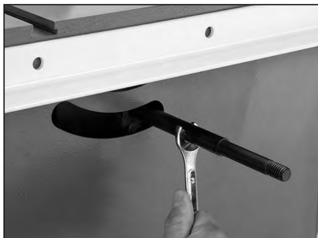
Figure 13. Installing the pivot shaft.
