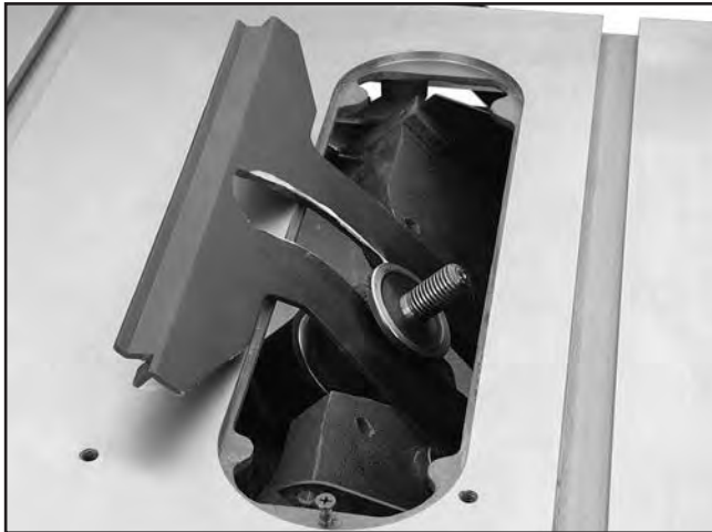
Figure 54. Removing the belt cover plate.
