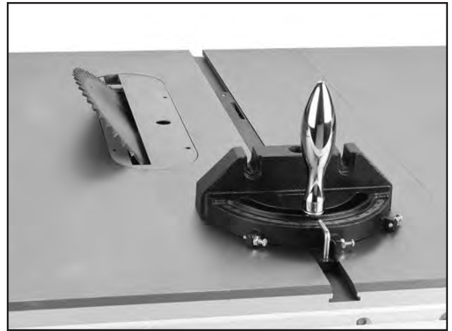
Figure 26. Blade tilted to 45° (guard removed for clarity).
